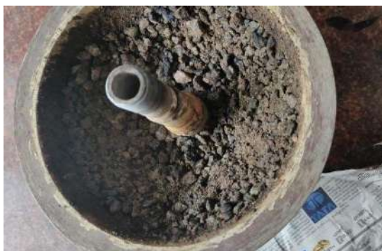
Fig. 3.4 Constituents of RAP after extraction In order to evaluate the cohesive strength of RAP modified base layers, samples are made by varying the WCO content and their ITS
