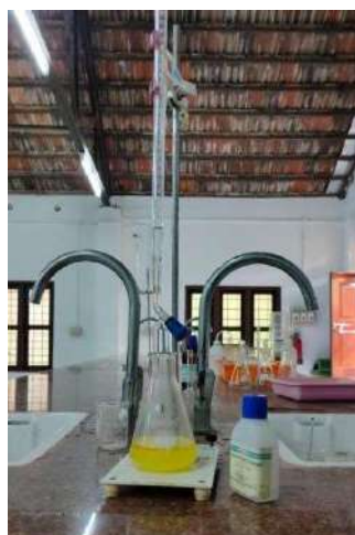
Fig. 3.2 Titration of oil sample against KOH
