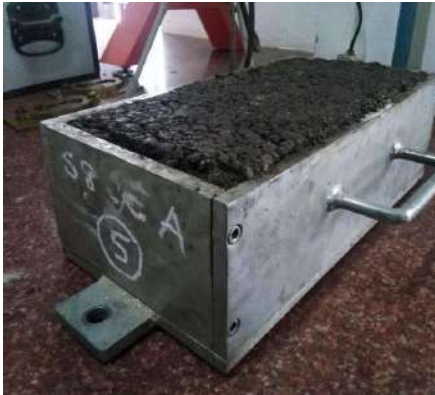
Fig. 3.11 Mould containing prepared Wheel Tracker Sample
