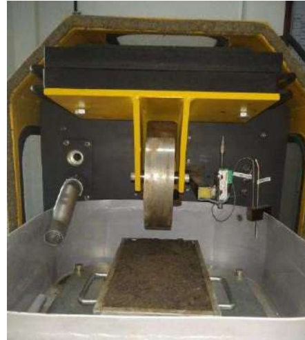
Fig. 3.12 Sample in Wheel Tracker for testing
