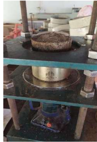
Fig. 3.10 ITS Sample Extraction
