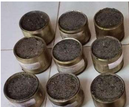
Fig. 3.9 Prepared ITS Samples
